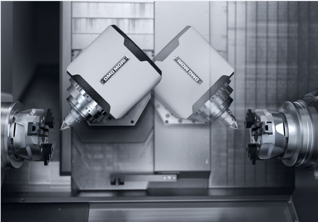
4 in 1 for full flexibility: Radial and axial machining with one tool – on both spindles
