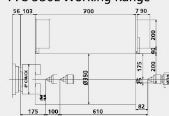
8-Position Turret Tool Interference Diagram (STD)
