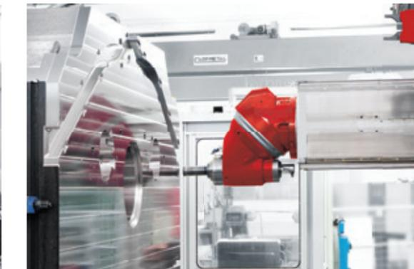
Mechanical machining of a mold by an automatic milling head 6000 rpm
