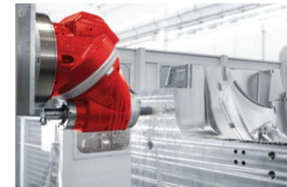
Mechanical machining of an injection mold for car bumper
