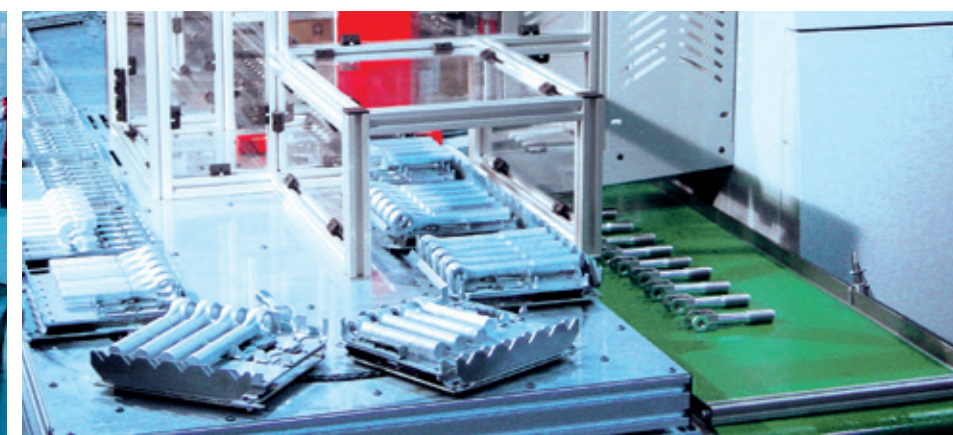
20-station pallet magazine with customer-specific pallets
