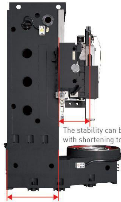
Thickness increased to guarantee structural rigidity.
