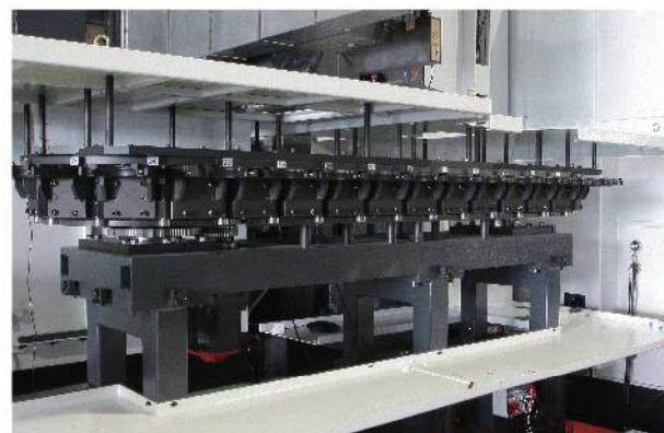
Tool magazine for 32, 48, 60 tool position
