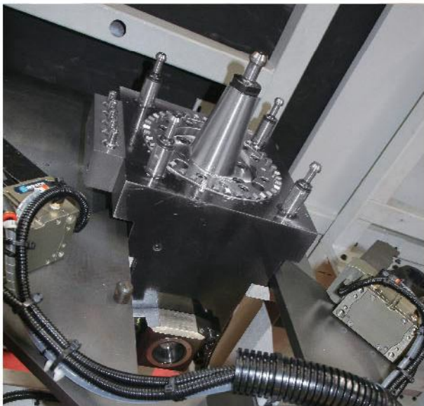
BT50 turning tool holder with 4 pull studs
