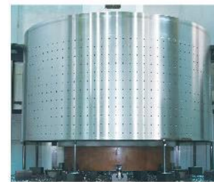
VTL3000ATC+C Wind power generator-rotor machining
